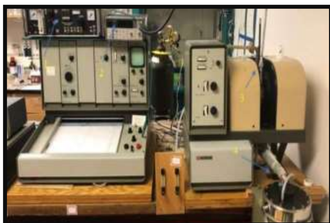
Figure 4. Setup of the Varian E-3 spectrometer (Dr. Petasis handout)
