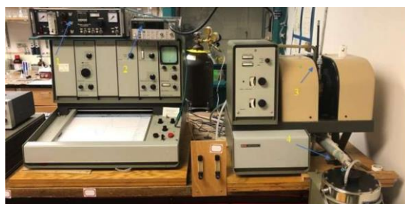
Figure 7. The Varian E-3 X-band spectrometer in Dr. Petasis' lab at Allegheny College. 1 corresponds to the temperature controller which displays the temperature and controls dry nitrogen flow, 2 is the universal counter that displays the microwave radiation parameters, 3 is the cavity where samples are placed and 4 is the liquid nitrogen dewar for supplying liquid nitrogen to the sample cavity during low temperature EPR scans.
